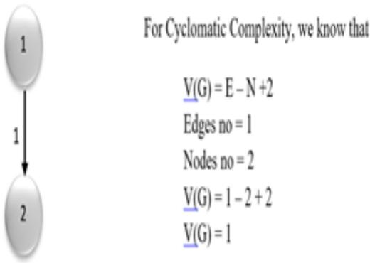
Figure 10. Flow Graph and CC of Plus Method that Add Byte type Values
