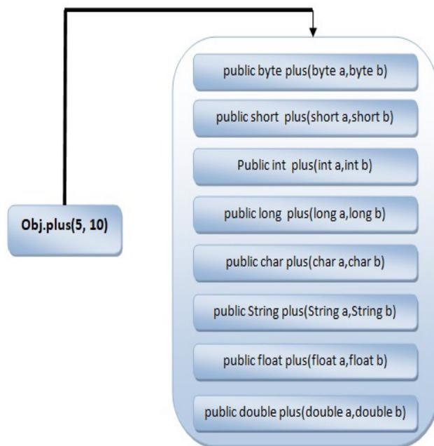
Figure 5. Depicted eight overloaded methods of plus class and calling way.
