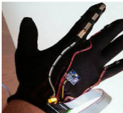
Fig. 2. Glove to control robotic arm
