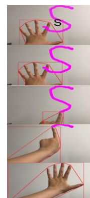
Figure 6: The output of the convex hull with tracking of the fingertip for the writing process
